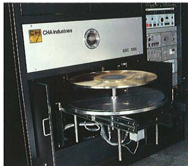
Substrate carrier rolls out for loading
