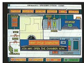
Process chamber before pump down
