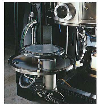
Substrate carrier swings out for loading
