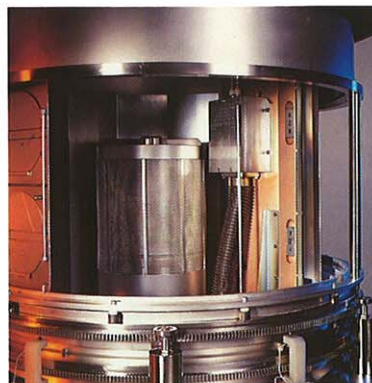
Backside of cathodes and condensible pump
