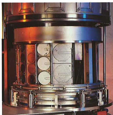
Mixed substrate sizes may be processed simultaneously (3" dia. & 4" dia. shown)
