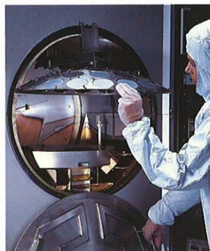
Operator loading lift off substrate carrier
